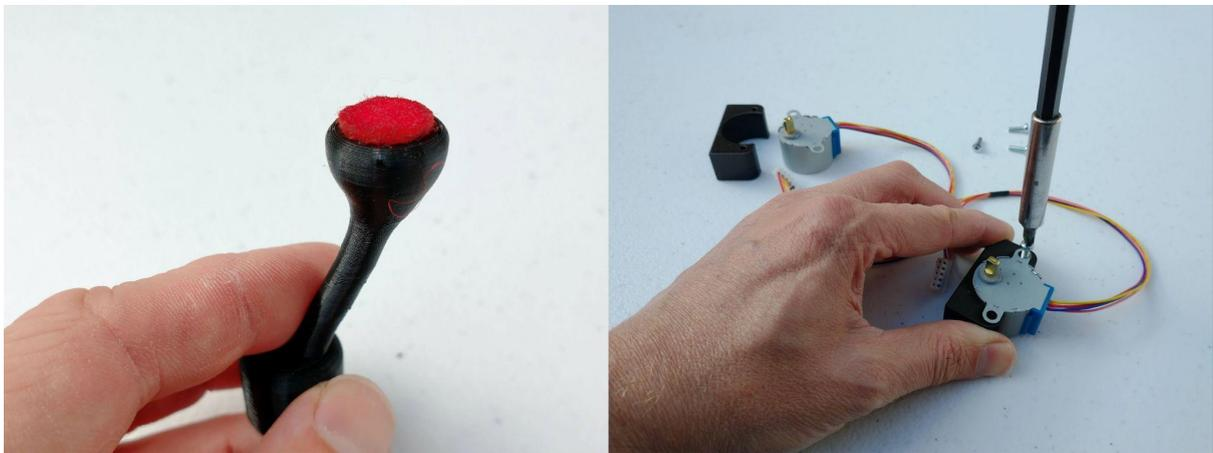
Next we need to attach the motors to the motor mounts. Simply place in the slot with the wires pointing away from the flat surface and screw in the shorter 10mm screws. The motor should not move, but be careful not to over tighten.
