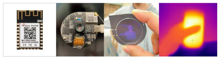
This IR Cam Application used RP2040, WizFi360 for Wi-Fi, and Bobcat's CMOS sensor for thermal images. Also, we used Arduino IDE for RP2040 and WizFi360 from Earle Philhower's library. For round screen GC9A01, we used the GFX library for Arduino.
