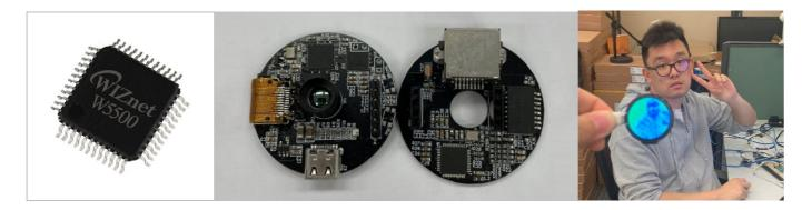
The Ethernet IR Cam using W5500 has similar hardware specifications as the Wi-Fi version using RP2040 + WizFi360.
